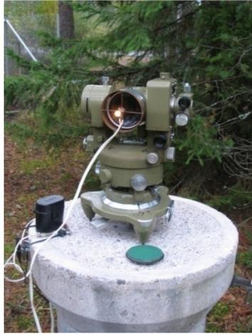
**Fig. 18.** Kern DKM3 theodolite with an autocollimation lamp on the theodolite pillar.
