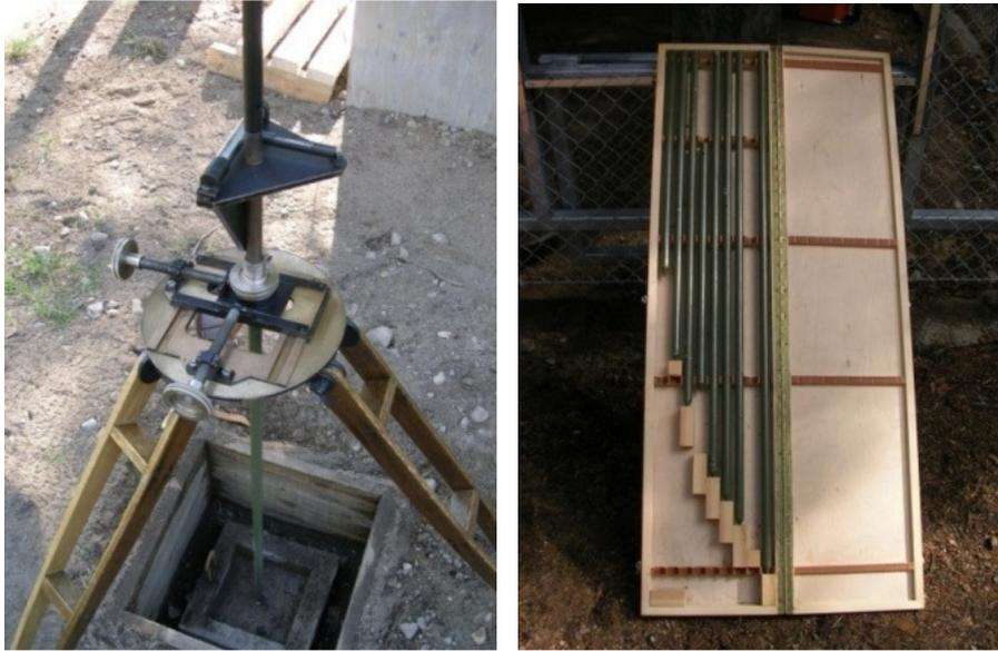
**Fig. 33.** A plumbing rod with two levels is adjusted above an underground marker using a special tripod with a stage slide system (left). A set of adaptor bars can be used to adjust the height of the plumbing rod (right).
