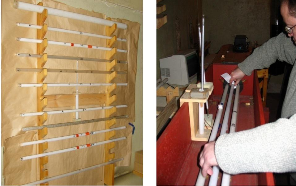
**Fig. 8.** Some of the most frequently used quartz gauges at Tuorla (left), and tuning a middle quartz gauge in the comparator “Saunapiano”. The side quartz gauges no. 63 and no. 64 are used to control the parallelism of the end planes.
