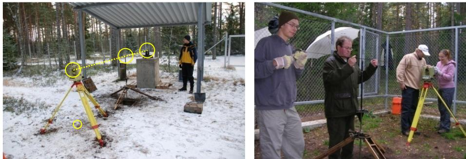
**Fig. 32.** Arrangements for projection measurements. The theodolite and the (top of the) adjustable plumbing rod are set up at about the same height with the mirror centre and perpendicular to the baseline (left). Marking the location of the theodolite with a wooden stick in the ground helps with finding the best location for later measurements. Four persons are needed for a properly performed tape measurement, two people holding the tape at a constant strain and two people reading it (right).
