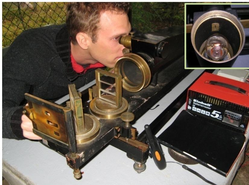
**Fig. 22.** Searching for interference fringes by adjusting the screen and turning the compensator glasses in front of the telescope. A detail of the lamp at the top right.
