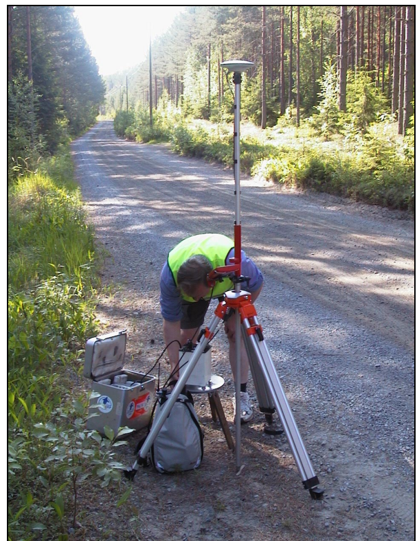
Fig. 7. Positioning of the gravity station by the RTK method. (Photo: Pasi Häkli)
