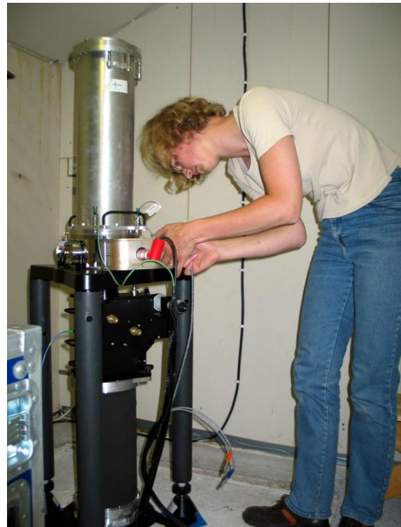
Fig. 13. Absolute gravity measurements at Vaasa GPS station. Photo Markku Poutanen.
