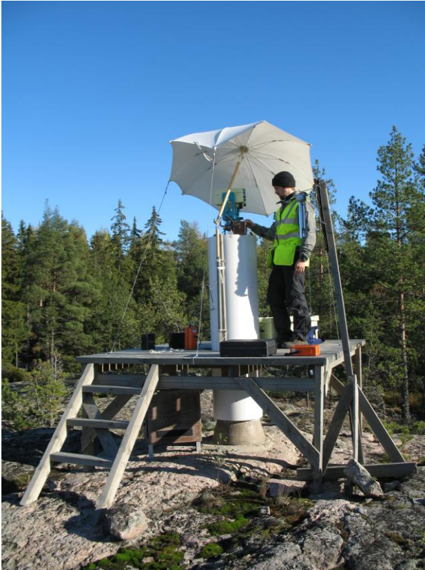
Fig. 20. EDM measurements at the Olkiluoto network. Photo Terhi Ahola.
