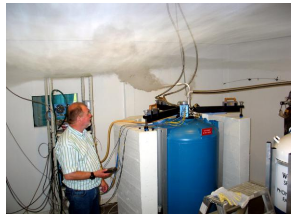
Fig. 15. Filling the Metsähovi superconducting gravimeter with liquid helium. Photo Markku Poutanen.
