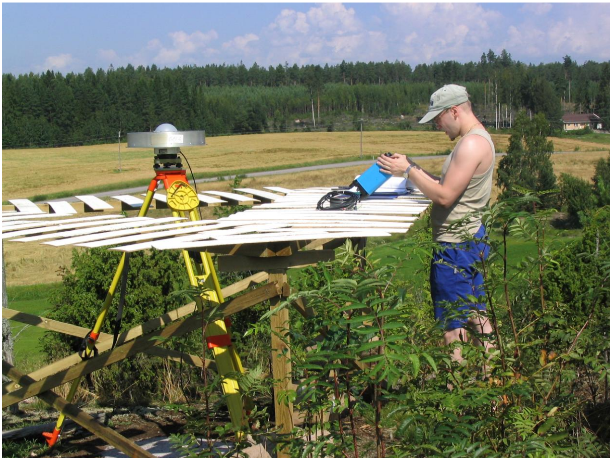
Fig. 30. Accuracy of the real time GPS was studied with field measurements in summer 2004. Photo Hannu Koivula.
