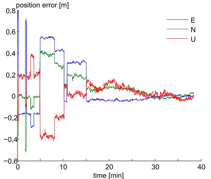
Fig. 6. Baseline estimation error in East, North, and Up components
