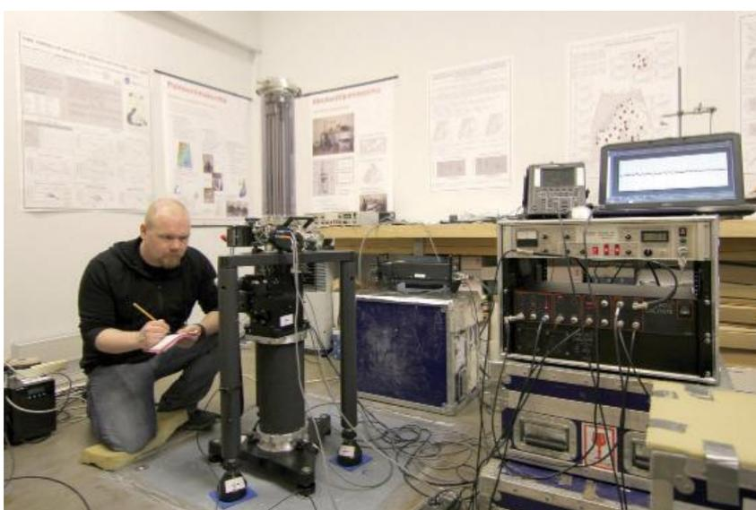
Figure 3. The absolute gravimeter FG5X-221 is based on a free fall experiment.
