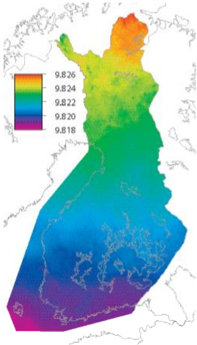
Figure 1. Acceleration of free fall in Finland, unit  $\text{m s}^{-2}$ .
