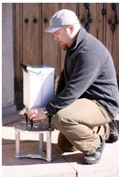
Figure 2. A measurement using a relative gravimeter.
