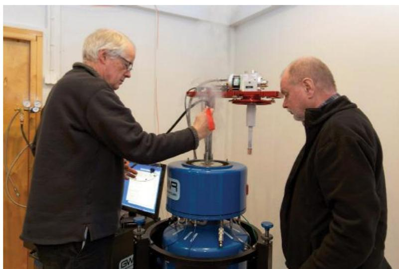
Figure 4. Superconducting gravimeter (Metsähovi, Kirkkonummi) registers even  $0.1 \text{ nm s}^{-2}$  variations in the acceleration of free fall.
