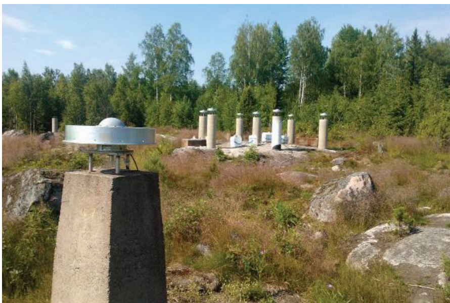
Figure 5. Research on the accuracy of GNSS antennas can be made at the test field of the Metsähovi observatory.
