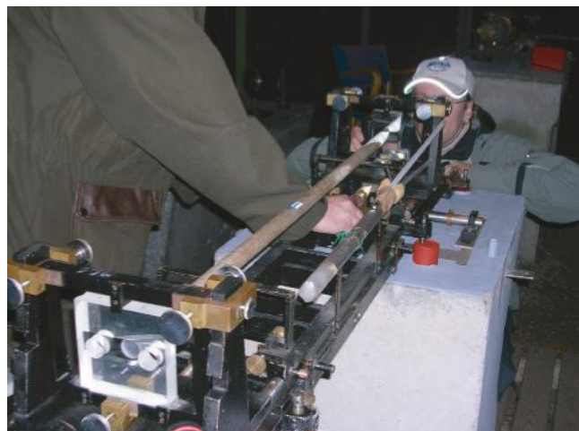
Figure 1 and 2. The Nummela standard baseline measured by using the Vaisälä comparator has been one of the most accurate and stable lengths over the past half decade.
