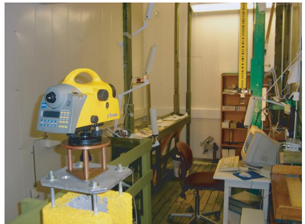
Figure 4. Calibration of a digital precise level instrument and system calibration of a barcode rod.
