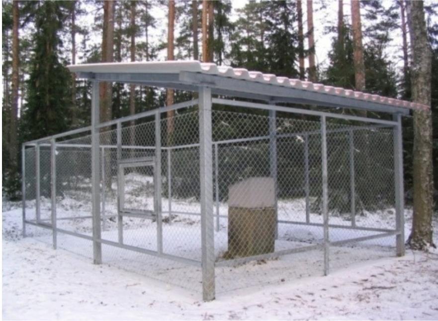
*Fig. 3. The new shelter at the 864-m observation pillar and underground marker.*
